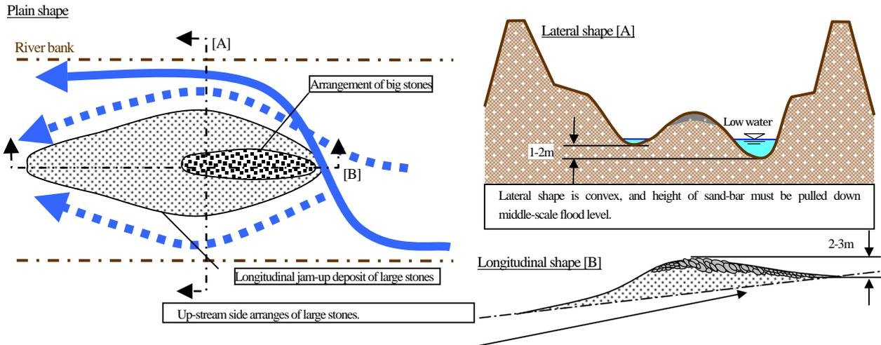
Figure 14. Restoration of double lanes meandering system
