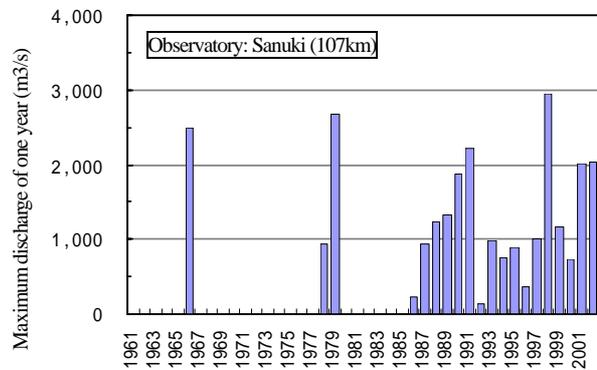
Figure 3. The rate of maximum discharge in Kinu-river (No data shows non-observation value.)
