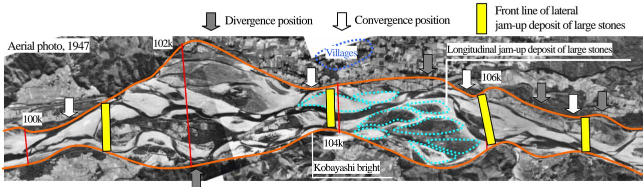
Photo 3. Divergence Convergence channel in Kinu river [ Aerial photo, 1947 before construction of levee ]
